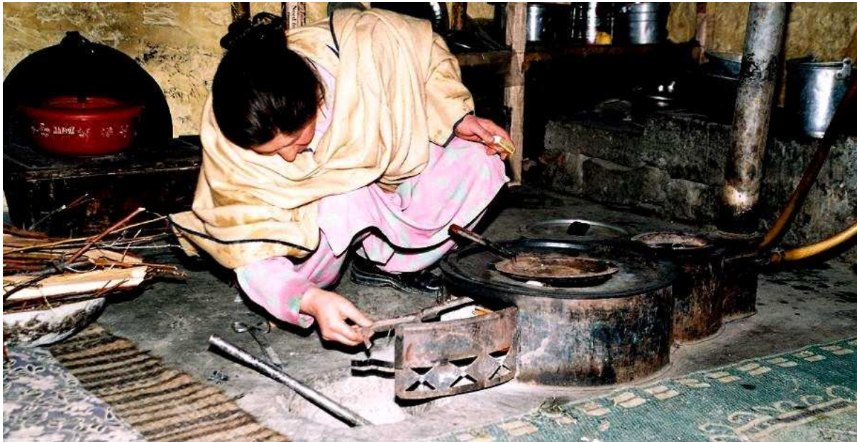
Fuel efficient BACIP stove improves smoke control in the house
